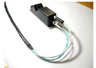
LC & M8 copper conductors connect to a single port remote indoor GatorLink
