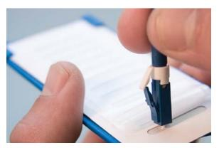
Today's optical networking components requiring minimal insertion loss and back reflections demand, quick reliable cleaning solutions. Fiber tips containing even trace amounts of debris not only suffer from power degradation but also an increased likelihood of permanent damage when mated.
