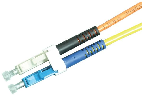
Our mode conditioning patch cords are custom made with any combination of ST, SC, LC, or MTRJ connectors at each end. A 9/125-singlemode fiber is offset to a multimode fiber on one leg while the other leg consists of a standard multimode fiber. The single mode/multimode side is plugged directly into the equipment. The duplex multimode side of the patch cord is plugged into the cable plant side.
